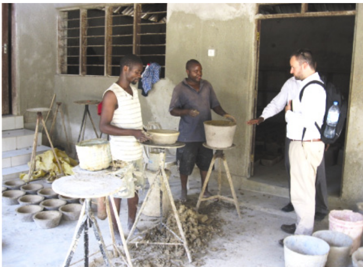
SEECO's production of clay liners for efficient cook stoves, Dar es Salaam, Sept. 2012
