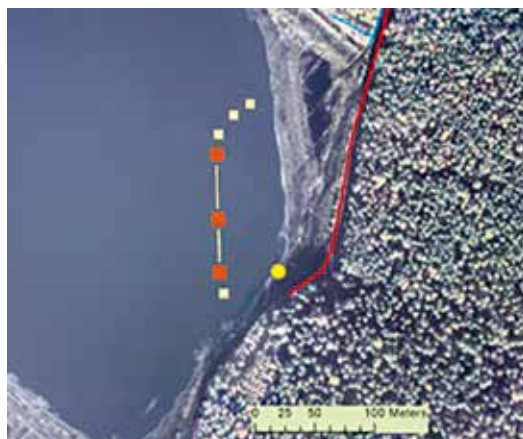
Figure 109. Arrangement of the floating islands on the eastern part of the post-excavating water basin. Red square (on the left picture) – a set of 12 islands (No. 1 in the figure to the right); white square – a set of 8 islands (2), lines – sets of 13 (3) and 10 (4) islands.
