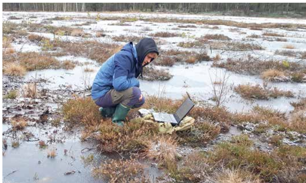
Figure 10. Water level monitoring well and the process of downloading the hydrological monitoring data in Sachara peatland (Lithuania). Photo: L. Sendžikaitė
