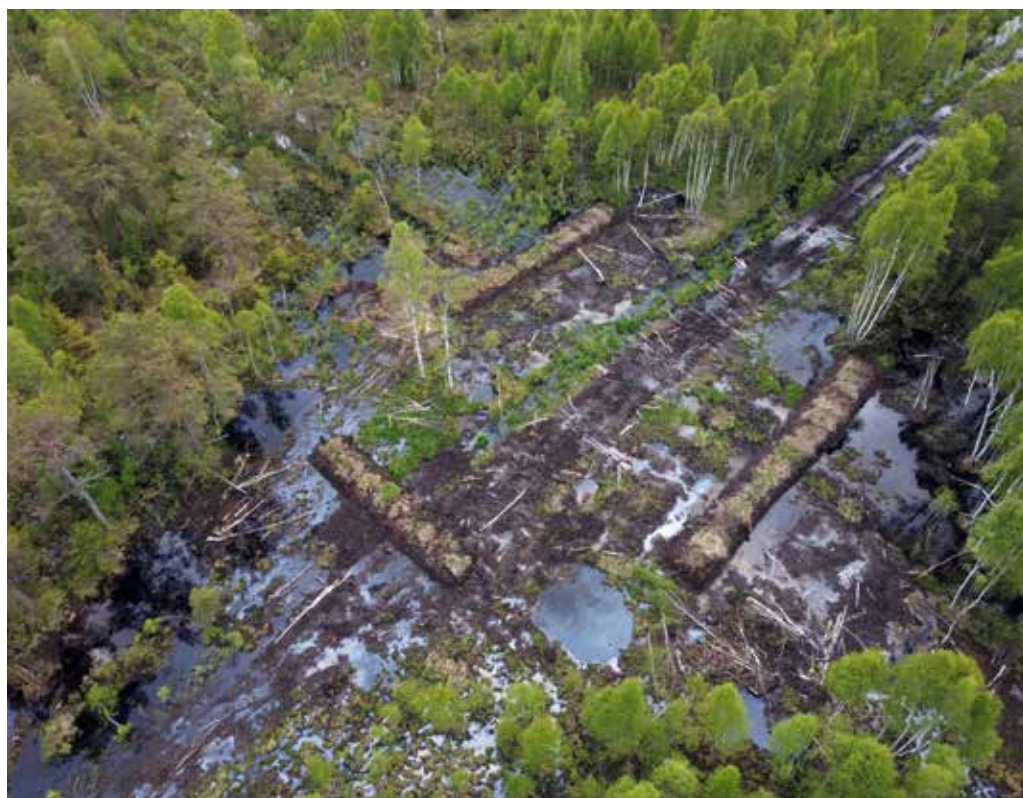
Figure 29. Aerial view of the ditch crossing in the eastern part of the Suursoo-Leidisoo restoration site in spring 2021 after the construction of the dams. The small pools are holes where peat was taken for dam building. Photo: R. Pajula.
