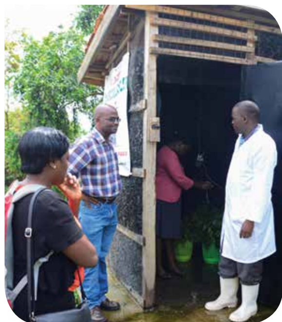
Charcoal cooler for vegetable storage experimented in Uganda, AIFV consortium.
